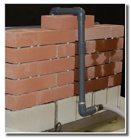
WCT units (on left) were spray bar tested with no mortar (just gaps) alongside a traditional block design (right) with a water flow rate equivalent to 180" of rain per hour for a half hour and then at a rate of 30" of rain for an additional 24 hours.
