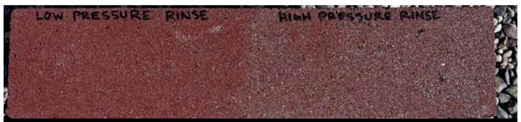
This Masonry Unit was cleaned with EaCo Chem NMD-80 using standard application methods, but the left side was rinsed using low water pressure and the right side was rinsed with high water pressure
