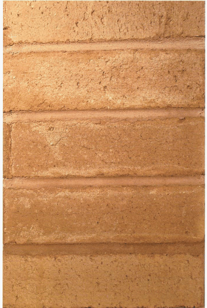
Fig. 3. In this example, a masonry prism was constructed using one batch of mortar. The top mortar joint was tooled immediately after placement of the unit. Remaining mortar joints were tooled at progressively greater time intervals and thus stiffer consistency. The relationship between mortar consistency when tooled and mortar color is quite apparent.
