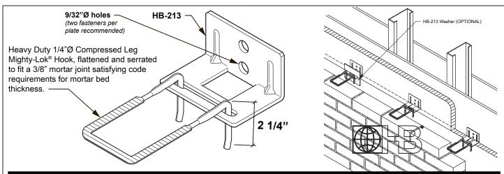
Hohmann & Barnard's Mighty-Lok Hook has been tested and designed to withstand over 290-lbf, in tension or compression, at maximum allowed offset (TMS 402/ACI 530 6.2.2.5.5.4) of 1¼" (disengagement of the pintle from the veneer anchor). These results exceed BIA recommendations and the capabilities of standard "round wire" hooks/pintles by over 100%, while maintaining the ASTM A1064/1064M wire specification.
