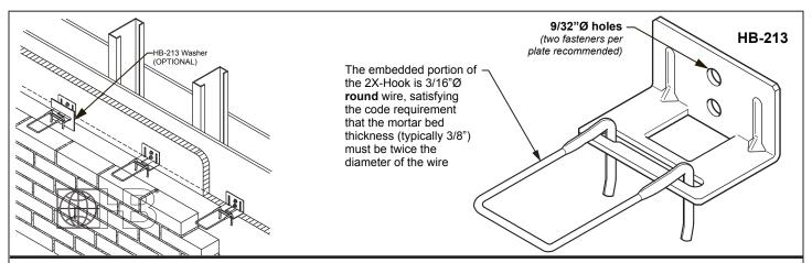
Hohmann & Barnard's 2X-Hook has been tested and designed to withstand over 200-lbf, in tension or compression, at maximum allowed offset (TMS 402/ACI 530 6.2.2.5.5.4) of 11/4" (disengagement of the pintle from the veneer anchor). These results exceed BIA recommendations and the capabilities of standard "round wire" hooks/pintles by over 100%, while maintaining the ASTM A1064/1064M wire specification.
