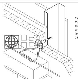
1½" Ø WASHER has been independently tested for ASTM E331 & ASTM 2357 performance standards, seals insulation, and helps secure insulation to backup; reduces or eliminates penetrations caused by insulation fasteners.
