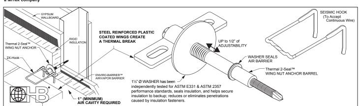
Hohmann & Barnard's 2X-Hook has been tested and designed to withstand over 200-lbf, in tension or compression, at maximum allowed offset (TMS 402/ACI 530 6.2.2.5.5.4) of 1¼" (disengagement of the pintle from the veneer anchor). These results exceed BIA recommendations and the capabilities of standard "round wire" hooks/pintles by over 100%, while maintaining the ASTM A1064/1064M wire specification.
